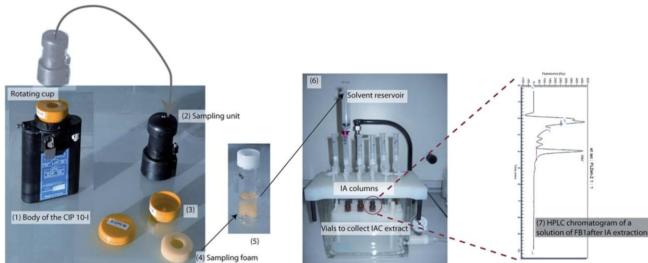
**Fig. 1** View of the CIP 10-I (1) during the laboratory analysis, its sampling unit dismantled (2), the rotating cup open (3) and the sampling foam removed from the cup (4). After the solvent extraction (5), the sample is applied to the IAC system (6). The IAC extract is then analyzed by HPLC-FLD (7).
