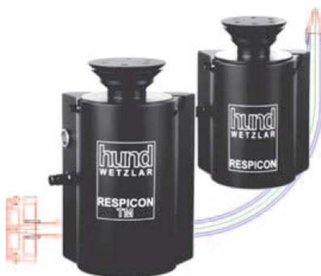
Figure 8 Respicon TM Respicon and virtual impactor
